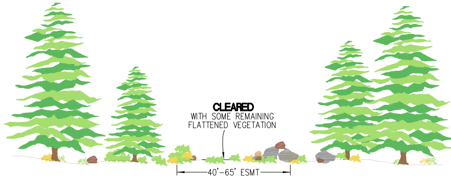
PROJECT CONSTRUCTION CONDITION
